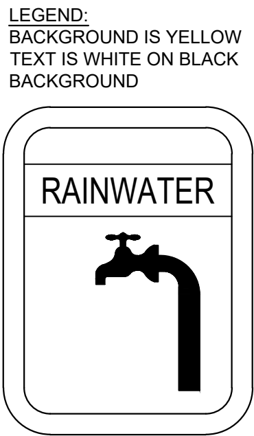
DETAIL 3 RAINWATER SIGN SCALE 1:10
